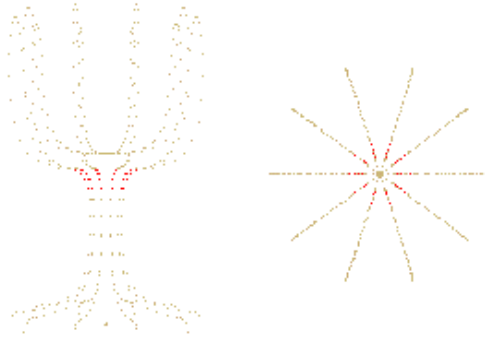
Figure 14: single zone/single value weights, obtained by the block(\zeta) -function (table 1). Observe the bolder dots in the zone from stem-to-cup. Left: front view, right: top view
