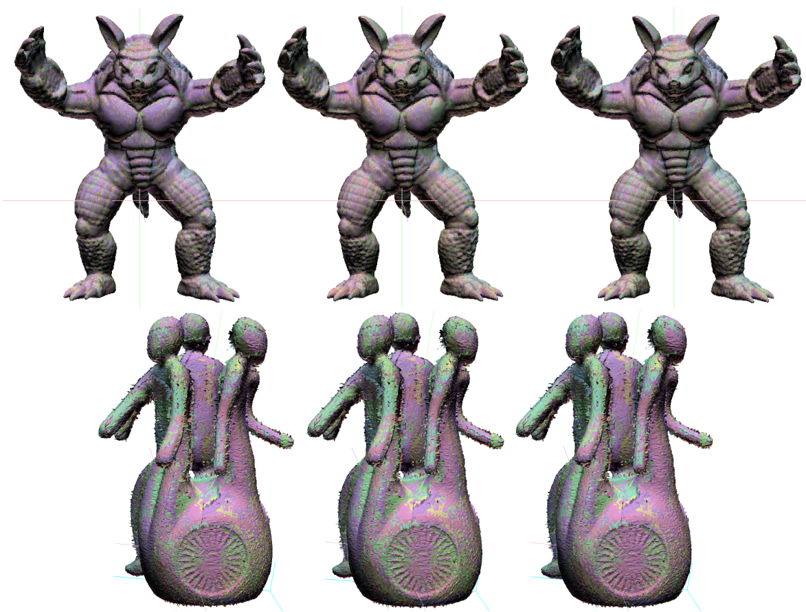
Figure 8: The results of the fine alignment. From left to right the results from MeshAlign, RapidForm and Scanalyze. The chest of the armadillo and the head of the memento show a difference in splotchiness.
