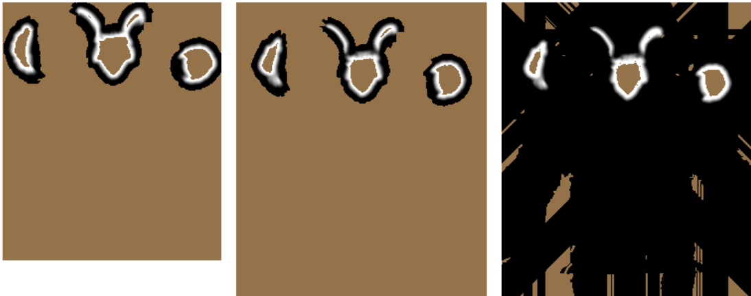
Figure 17: Slices of VripPack's volumetric distance field grid created for the armadillo (head and arms), showing the signed distance and weight functions in 2D (brown=unseen, black=empty, [black, white]=near the surface mesh). From left to right: A slice with tight bounding box, a slice with a larger bounding box, and a slice showing space carving.
