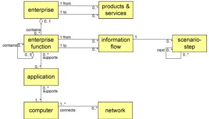
Fig. 1. The metamodel of the Enterprise Architecture Modeling method (EAM)
