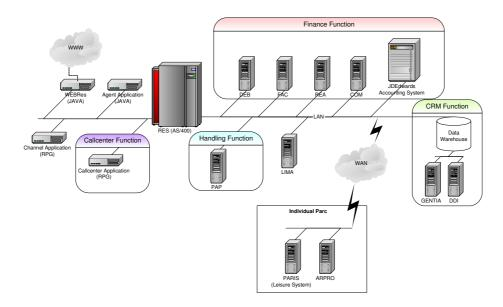
Fig. 7. Example System Infrastructure Diagram, a mixture of platforms at Center Parcs
