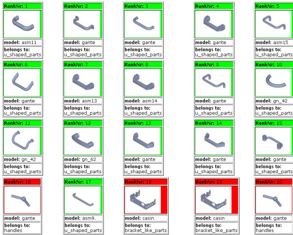
Figure 13. Query 40 from u_shaped_parts class with run 1. aMRG resolution is 4, and the graph matching approach is fully topologic. The class is very well retrieved.
