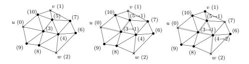
Figure 3: From left to right: a terrain with three local minima: at u, v and w; a breaching path from v to u; a breaching graph of minimum cost that connects u, v and w.
