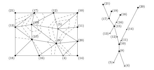
Figure 1: Left: example of a terrain showing the elevation of the vertices (between parenthesis) and some of the contour lines. Right: the augmented contour tree of the terrain.
