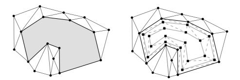
Figure 7: Left: a face of the input graph (in gray) that needs to be triangulated to turn the graph into a valid terrain. Right: a series of smaller copies of the face, two in the example, are created and triangulated; the center hole still not triangulated can be triangulated in any way.
