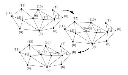
Figure 2: Removing the local minimum of height 4 by lowering. Top: initial heights (between parenthesis). The change in height of the lowered vertices is shown with an arrow. Middle and bottom: first a vertex is lowered from 6 to 3, turning it into a new local minimum. To remove it, a neighboring vertex is lowered from 7 to 2. A breaching path from the vertex of height 4 to the one of height 1 is highlighted in gray.
