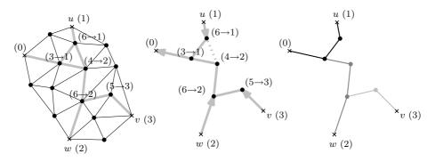
Figure 4: Left: terrain with four local minima, together with the breaching graph of an optimal solution (only the relevant heights are shown). Center: the breaching graph seen as a tree, with the removal direction shown. Right: payment of the lowering the intermediate vertices. The black vertices are paid by u, the medium gray vertices by w, and the light gray vertex by v.
