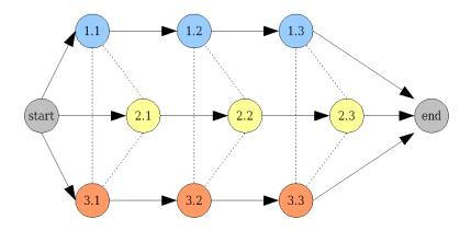
Figure 2: A disjunctive graph representing a JSSP instance.
