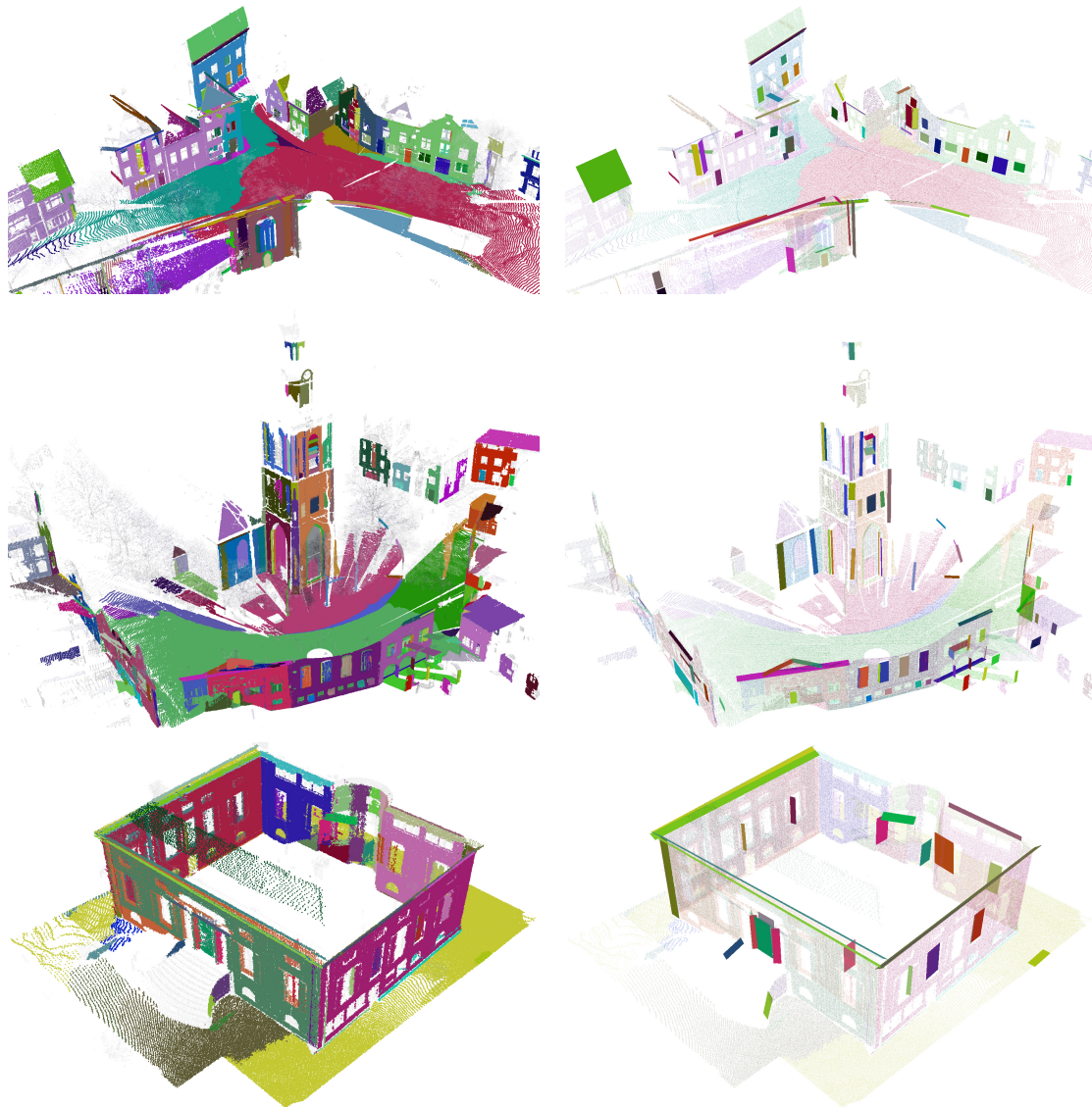
Figure 12: Some examples of our ground-based data sets. The left figures show the point data colored by cluster; Points that could not be assigned to a cluster are shown transparent black. The right figures emphasize the rectangular surfaces. All rectangles shown are \delta -covered. If there is a \delta -covered rectangle that fits the intersection with a neighboring surface, this rectangle is shown. Otherwise, rectangles with a horizontal edge are preferred; if there is no \delta -covered rectangle with a horizontal edge, an arbitrary \delta -covered rectangle is shown. For these examples, \delta is set to 40 cm.
