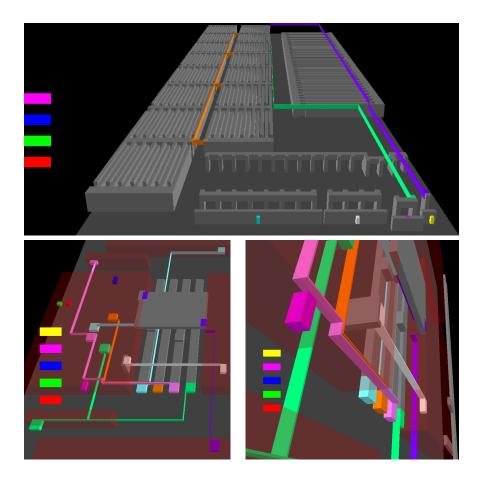
Figure 1: Screenshots from the demonstration at NXP, Eindhoven. The top picture shows generated routing for the tunedCap circuit and the bottom two pictures show routing for difInvStage. Both these circuits consist of 5 layers.
