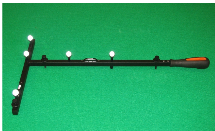
Figure 5: Image of the Vicon calibration wand.
