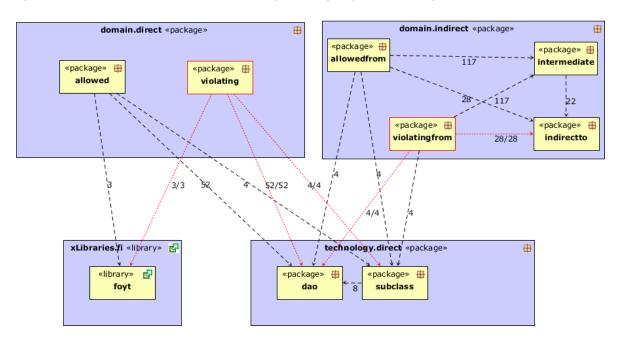
To measure the false positive rate of the ACC tools, 64 cases are aimed at the detection of false positives. Packages domain.allowed and domain.indirect.allowedfrom contain copies of the classes in the corresponding violating packages, so dependencies to the same to-classes are contained. Since no architectural rule constrains the classes in the "allowed" packages, reported violations of these classes are qualified as false positives.
