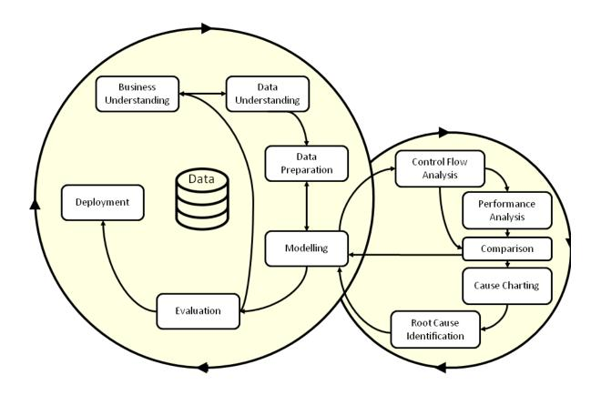
Figure 6. The CRISP-DM extension for Root Cause Analysis of Data Interoperability Problems (CIRCA-DIPS) conceptual method.
